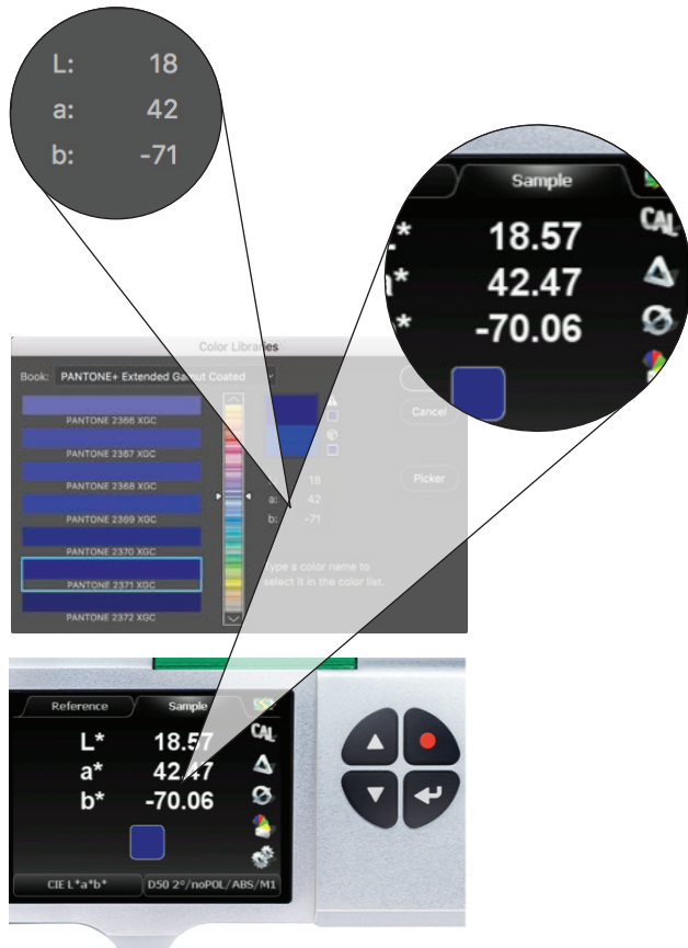
Figure: L^*a^*b^* values between Photoshop and measured values from a Pantone Extended Gamut Guide swatch book are nearly identical. Would you have achieved such accuracy in your older swatch books?
