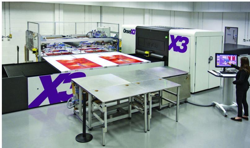
Figure 2: Inca Onset X3 for Multi-Pass Printing of Corrugated Board
