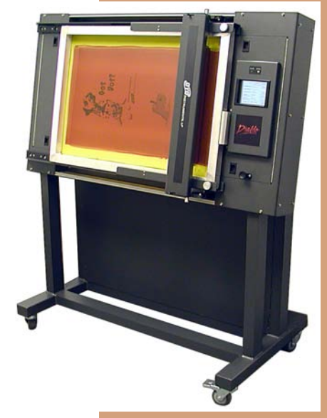
Figure 8: The Diablo from OYO Instruments LP is the industry's first computer to screen device using thermal transfer technology.
