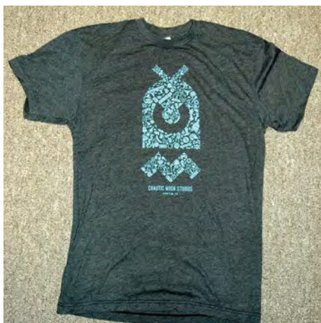
Photo 2: Here the effects of printing a discharge onto a 50/50 cotton / Poly blend are shown. (Garment courtesy of Real Thread, Orlando FL)
