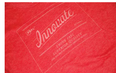
Photo 5: Here you see the screen image where the cotton fibers have been washed away following the printing and curing process. (Garment courtesy of Real Thread, Orlando FL.)
