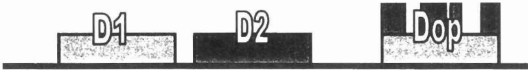
Figure 1. Ink trapping: when printed directly on paper, both the first-down (D1) and second-down ink (D2) form a uniform film. When they are overprinted (Dop) though, the second down ink film resembles a halftoned image.
