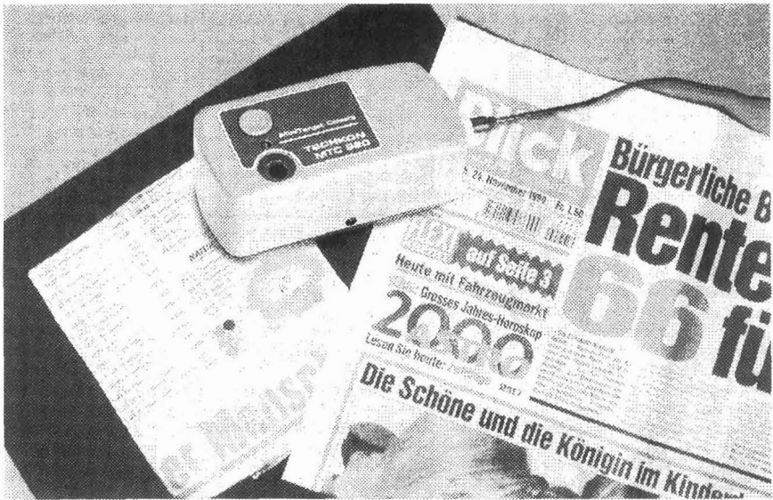
Fig. 6: Prototype of an easy to use handheld device. The device will be placed on top of the MiniTarget. A measurement is carried out by pushing a button. The results will be shown on the computer screen.
