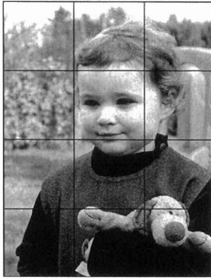
Figure 7. A tile (mask) with threshold values is placed over the image and repeated in horizontal and vertical direction allowing a very fast rendering.
