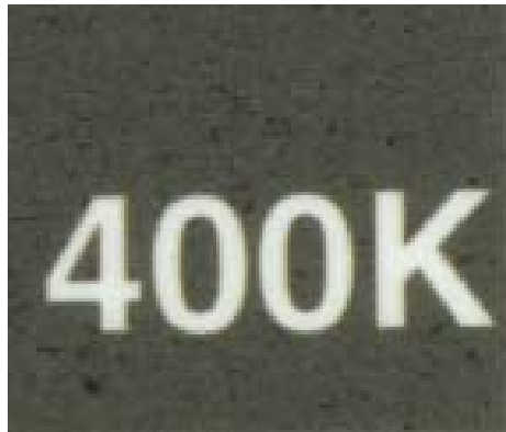
Figure 7: A 2000 ppi image showing the lower right corner of a four color black offset print showing the name of the image. Note below the “4” is a black speck. This speck was visibly identified as a high gloss area reflecting low angle incident angel light. The area surrounding it did not. Fig. 8 shows this speck enhanced.
