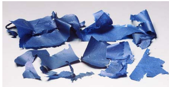
Figure 7: "Sheets" of lint - mostly ray cells - peeled from the blanket of a heatset offset press [2].
