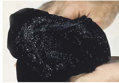
Figure 3: A “black velvet cloth” showing lint fibres collected after contact with the moving paper.
