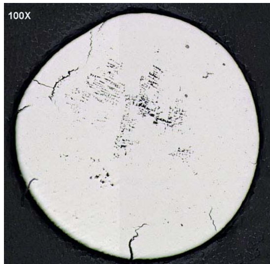
Figure 15: Cross-section of a steel pellet used to grind ink (diameter ~2mm).
