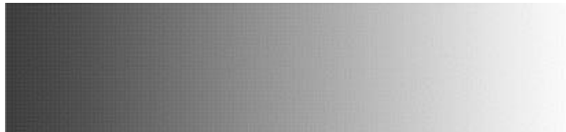
Figure 6. Tone wedge where 2 sub dots are removed for a smooth tone transition.
