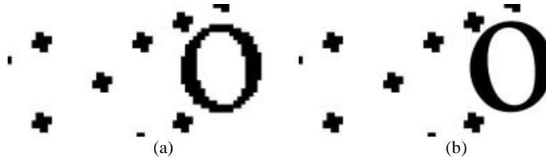
Figure 13. Image (a) of an expanded and shaved single resolution file and (b) a dual resolution file where just one part is expanded and shaved and the other part was screened at higher resolution.
