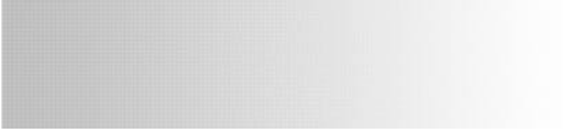
Figure 7. Same tone wedge as Figure 6 showing the results of an excessive shaving where 50% of sub dots were removed for an overall loss of contrast giving a low key result.
