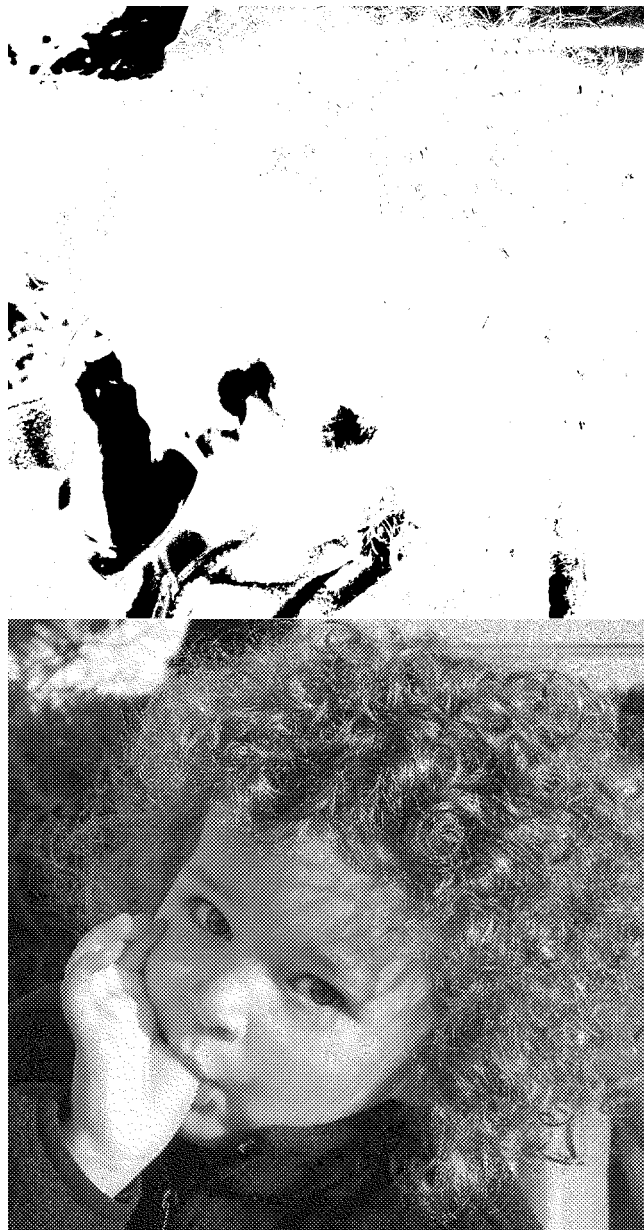
Figure 11. Hybrid screened image (bottom) obtained by applying AM to midtones (10% - 90%, white in top image) and FM in highlight and shadows (black in top image).
