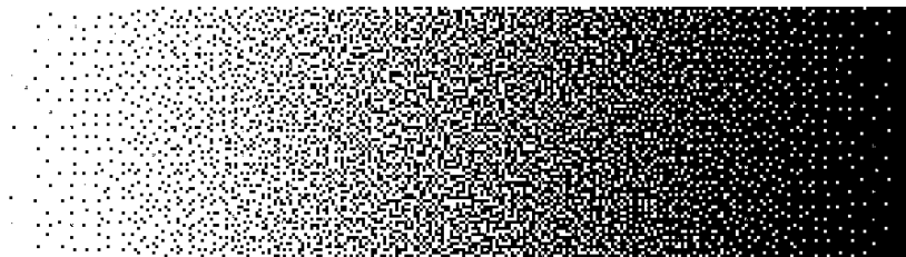
Figure 9. Agfa's Cristal Raster applied to a grey vignette. Around the 30% too many dots have to be placed to keep them apart. So some dots will start clustering. This amplifies the graininess of the FM screen.
