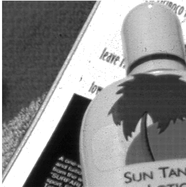
Figure 3: AM-halftoned image in 600 dpi and 100 lpi. The printing method is supposed not to be able to print the dots sufficiently small to manage the gray tones under 11%.
