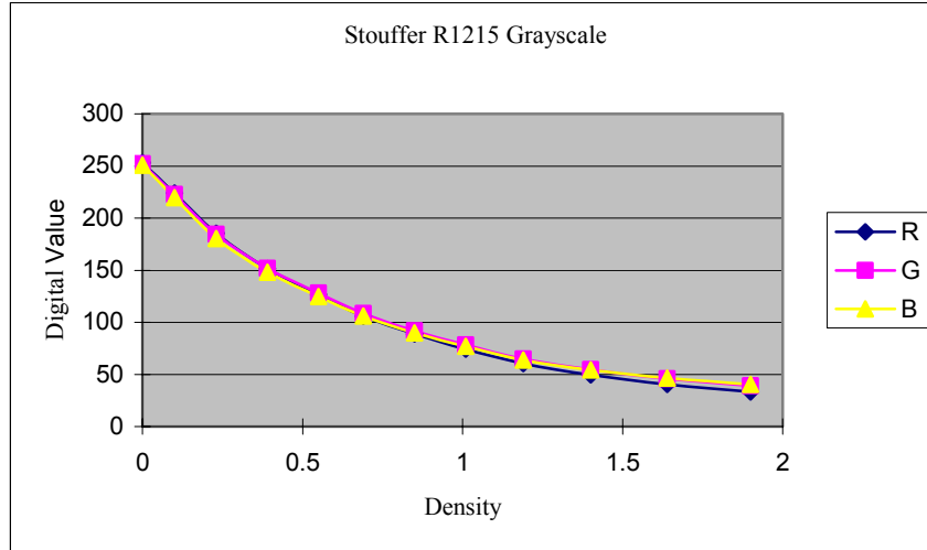
Figure 1: RGB digital values of Stouffer R1215 grayscale scanner by HP Scanjet 7400C with no auto adjustment.
