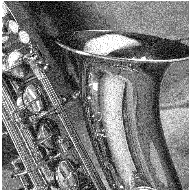
Figure 10: The test image is halftoned by the non-modified Error Diffusion method and printed at 300 dpi. The original image is not compensated for dot gain.
