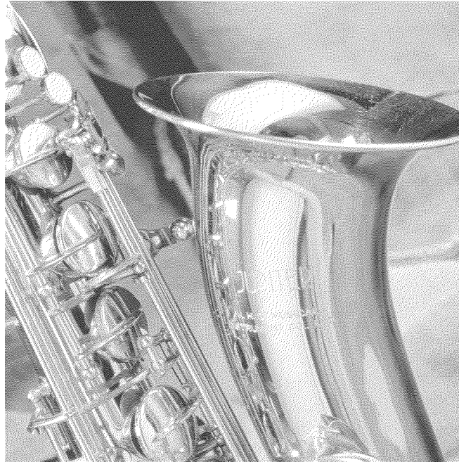
Figure 11: The compensated test image is halftoned by the non-modified Error Diffusion method and printed at 300 dpi. The original image is compensated for dot gain.
