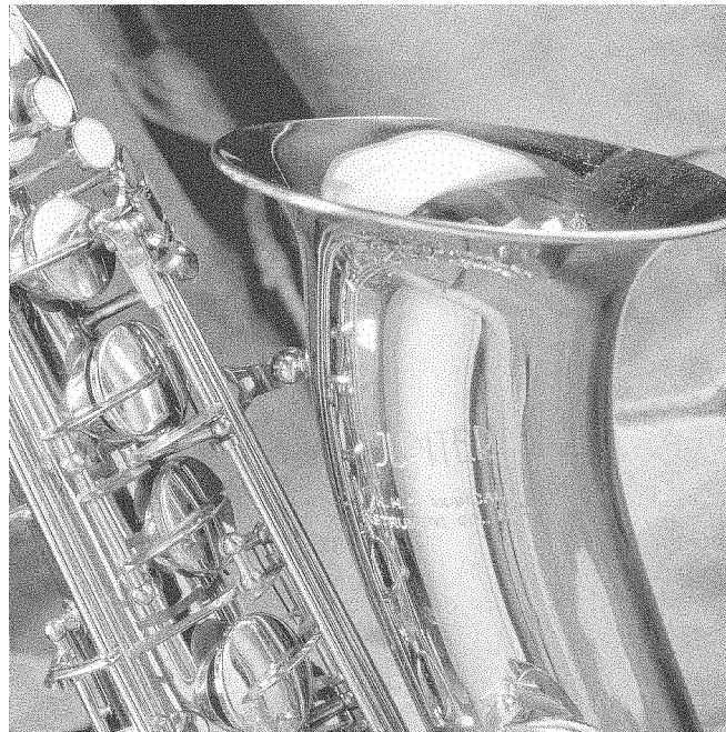
Figure 8: The compensated test image is halftoned by the presented FM method and printed at 300 dpi . The original image is compensated for dot gain by using the curve in Figure 1.
