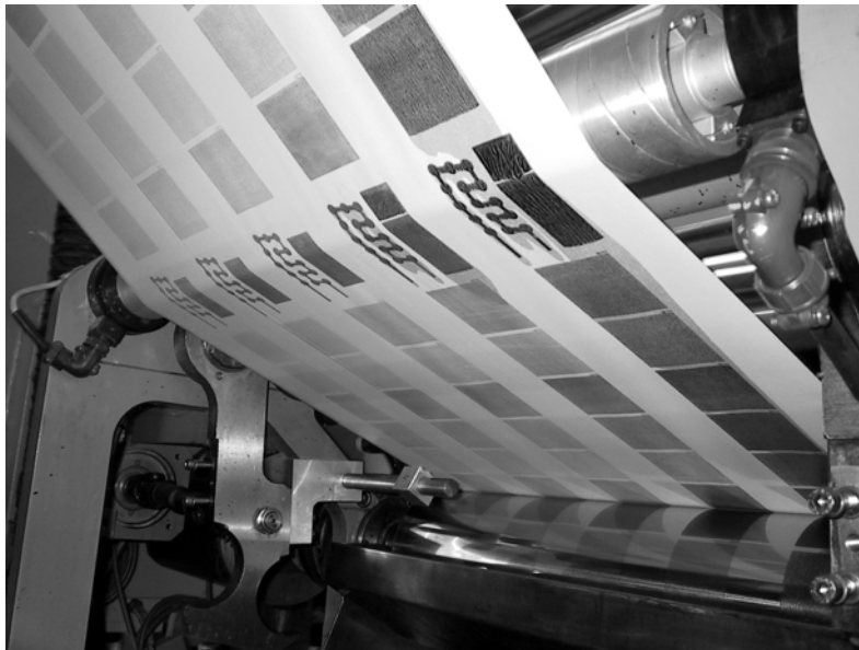
Figure 9. Reel-to-reel printed conductive polymer structures gravure, Metso Pilot gravure (Makela, 2003)
