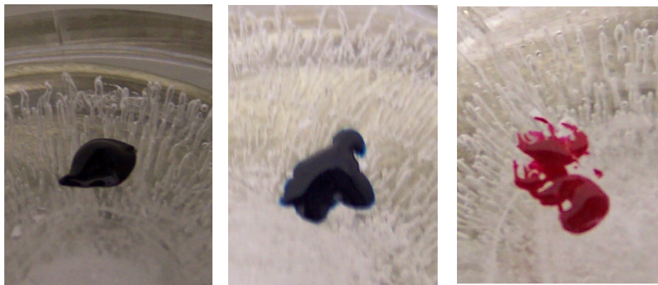
Figure 8. Photographs of the transfer of ink onto ice surface at -7\text{ }^{\circ}\text{C} using the glass rod dabbing method (See Figure 3). From left to right are black, cyan and magenta inks.
