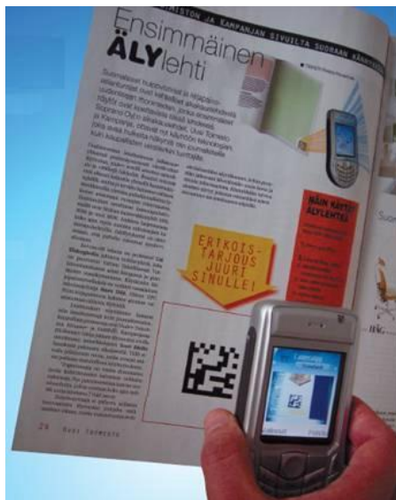
Figure 2. A smart magazine. A 2D code can be read by a mobile phone and additional information is automatically downloaded from the Internet.
