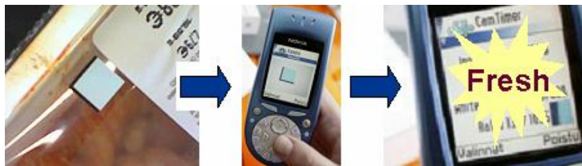
Figure 7. VTT's internationally patented inkjet printed food quality indicator system. A consumer can check the freshness of a food product by taking a picture of an inkjet printed food quality indicator. After the frame is taken, the mobile phone software automatically interprets the color information and informs the user of the status of the product.
