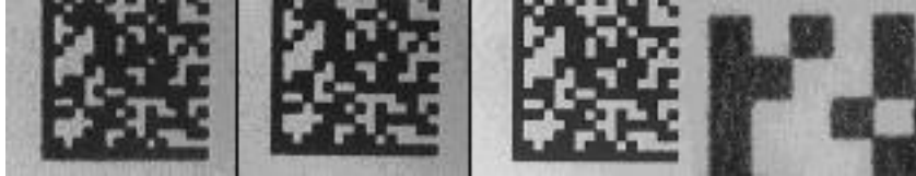
Figure 4. Two dimensional bar codes on different papers. From left: newsprint, SC paper, LWC paper and coated paper. Cell size is 250\ \mu\text{m} .
