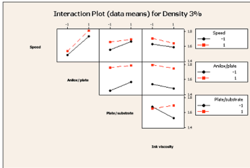
Figure 10 The interaction plot for print density for the analogue plate results
