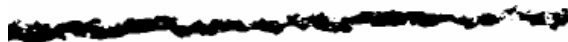
Fig.6a and 6b: Cross section (optical microscopy) of a black toner's layer after fusing on paper. Below (Fig.6.b) the binarization of this layer is presented. (EFPG)
