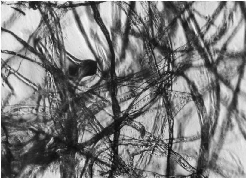
Figure 4. Cellulose fibers, magnified 150 \times .
