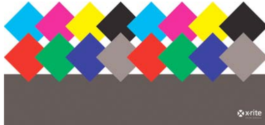
Figure 5. A color test form consisting of solids and 2- and 3-color overprints can be used to set optimum printer heat. This image facilitates observation of ink mottling, vertical and horizontal banding
