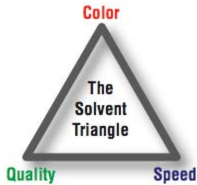
Figure 4. Ecosolvent inkjet printing involves a tradeoff between color, quality, and speed. Maximum color density (therefore, gamut) may be achieved at maximum heater temperature, but media buckling and the resultant vertical banding will adversely impact quality. Likewise, the highest color density is achieved at lower print speeds, which adversely affect throughput. Maximum quality (resolution, sharpness, freedom from artifacts) will be achieved with reduced ink density and speed.
