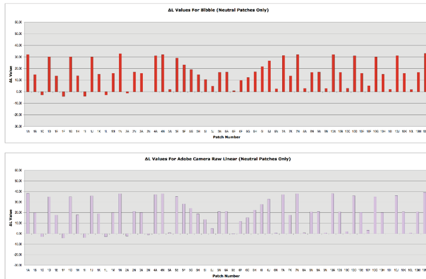
Figure 6: Charts showing the \Delta L value for neutral patches in Bibble Pro and Adobe Camera Raw Linear. Patch numbers were used as the x-axis as a constant to compare colorimetric differences.
