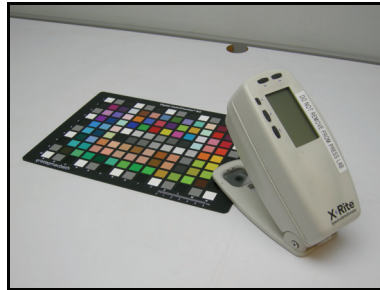
Figure 2: GretagMacbeth Digital ColorChecker SG and X-Rite 530 Spectrodensitometer.
