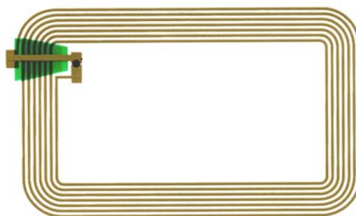
Figure 2. Antenna design (13.56MHz, 45mm x 76mm) for the study
