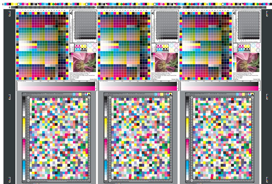
Figure 2, One of the two test forms containing the randomized RIT 100 Steps Charts
