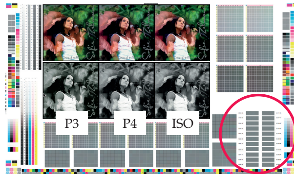
Figure 26: The new test form for Printing 5, the red circle shows the hidden words inside the patches.
