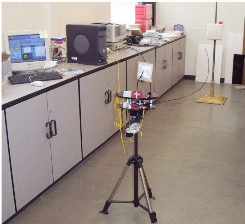
Figure 14. Laboratory RF Antenna Measurement set up.
