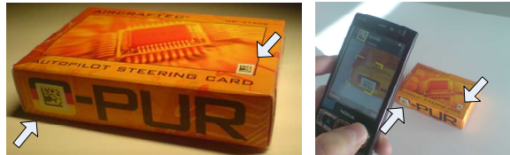
Figure 1: An exemplary product package supplied with a mobile tag with integrated anti-counterfeiting features
