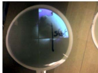
Typical Error short through the first dielectric layer
