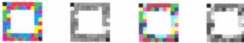
Figure 9. Color-optimized barcodes, created by HPLabs, and their copies. (Source: Simske et al. (2009)).
