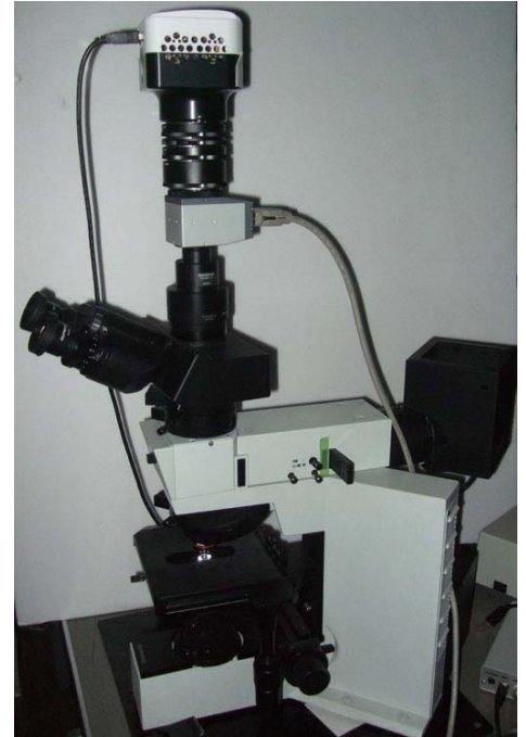
Figure 5. The reflection optical microscope attached with a liquid crystal tunable filter (LCTF).
