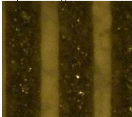
Figure 33. A magnified view of the print directional line (300 lpi).
