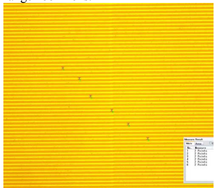
Figure 4. 10.58 m\mu horizontal line (measured width 10.5 \mu\text{m} ).
