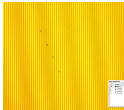
Figure 5. 10.58 m\mu vertical line (measured width 9.6 \mu\text{m} ).
