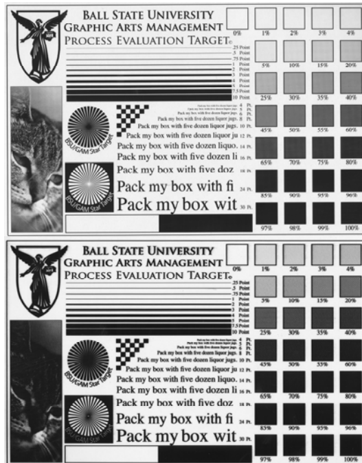
Figure 2. Comparison of photographic (left) and inkjet-printed (right) films.
