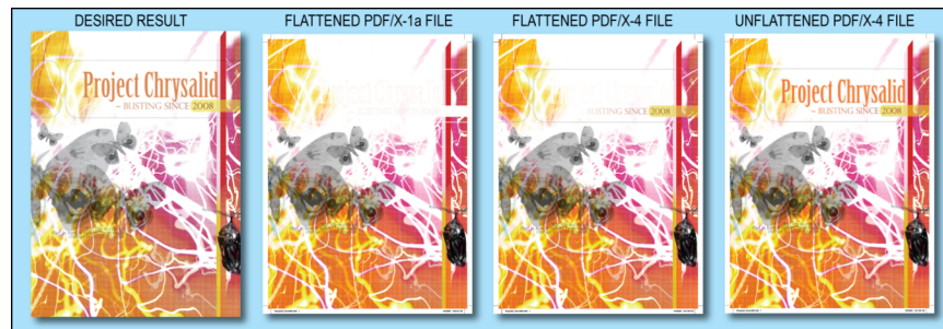
Figure 5. Comparison of flattening results on page one of the test form. Note that both the PDF/X-1a and PDF/X-4 files rendered incorrectly when flattening was applied.
