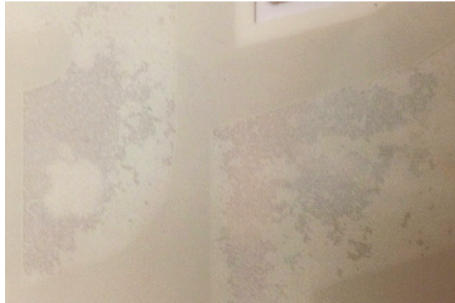
Figure 6: Poor adhesion appeared between phosphor ink and ITO surface.
