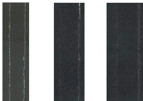
Figure 1: Printed and folded paperboards with aqueous coating applied. Folding lines were scanned with an Epson scanner. The left one was printed with Ricoh C900S. The paperboard was not corona treated. The middle one was printed with HP Indigo 3050 on the untreated paperboard. The right one was printed with HP Indigo 3050 on the corona treated paperboard.
