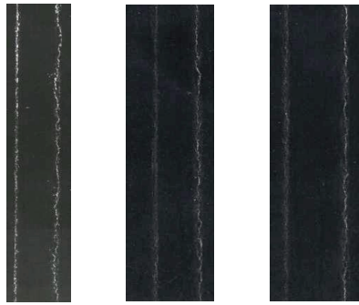
Figure 2: Printed and folded paperboards without aqueous coating applied. Folding lines were scanned with an Epson scanner. The left one was printed with Ricoh C900S. The paperboard was not corona treated. The middle one was printed with HP Indigo 3050 on the untreated paperboard. The right one was printed with HP Indigo 3050 on the corona treated paperboard.
