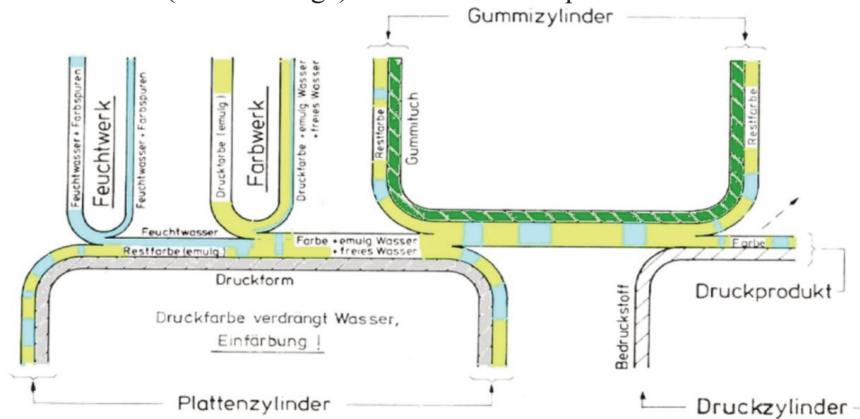
Figure 5: Systematic of the water flow in the printing system
