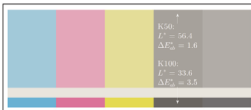
Figure 11: Example 4 - solids and 20%, optimized image. The system makes a compromise to balance the errors between the solids and the mid-tones.
