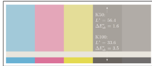
Figure 9: Example 3 - solids and 50%, optimized image. The system makes a compromise to balance the errors between the solids and the mid-tones.
