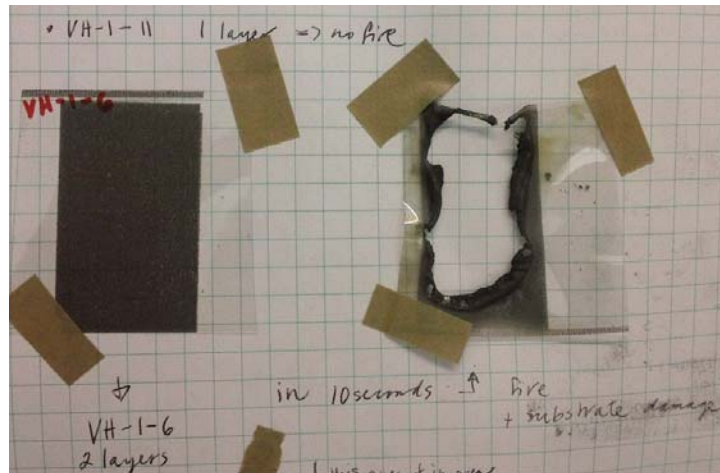
Figure 8. Susceptor constructed out of 2 layers on the left. Same susceptor after 10 seconds in microwave oven.
