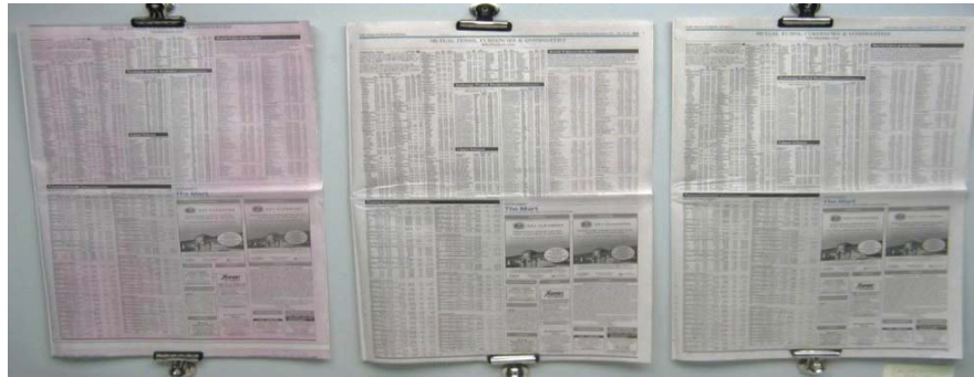
Figure 10: Examples of toning - Heavy toning on the left, light toning in the middle, and no toning on the right
