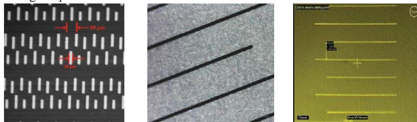
Figure 9: Stencils can be used for printing. Only simple shape of features can be imaged.
