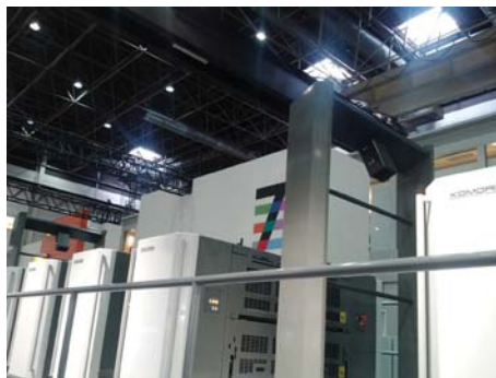
Figure 11: Komori's PQA-S: Inline quality check + inline density control
