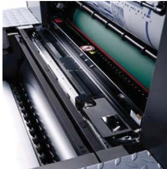
Figure 10: Heidelberg's Prinect Inpress Control Spectrophotometer.
