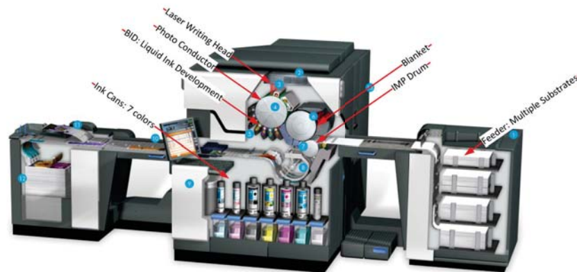
Figure 1: Liquid Ink Electrophotography
