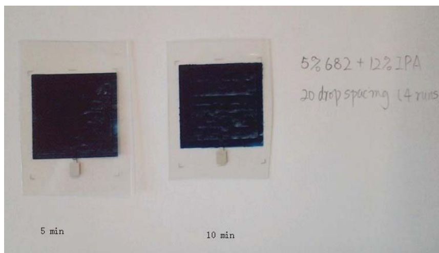
Figure 7. Insulator layer after UVO treatment, ink with 5% J682+12%IPA
