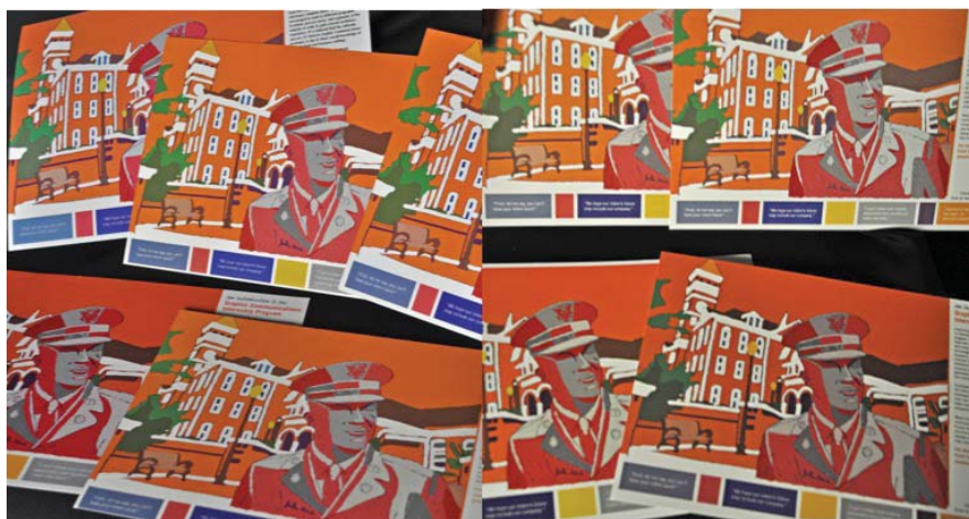
Figure 17: Samples received from multiple print providers, the image on the left are from the RGB color space prints and the samples on the right are CMYK, with GRACoL profile embedded
