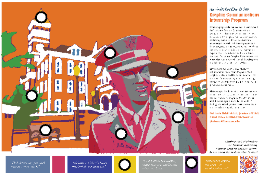
Figure 2: Vector art postcard with 10 measurable patches of spot colors from the X-Rite ColorChecker target; patches indicated by white circles with black outline
