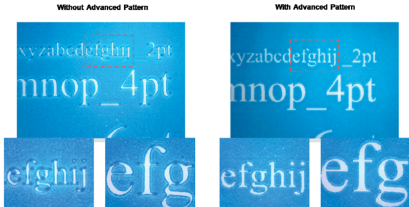
Figure 7 – Images showing at 200X magnification the impact of Advanced Edge Definition (AED) with fine text reverses for solvent based ink on film
