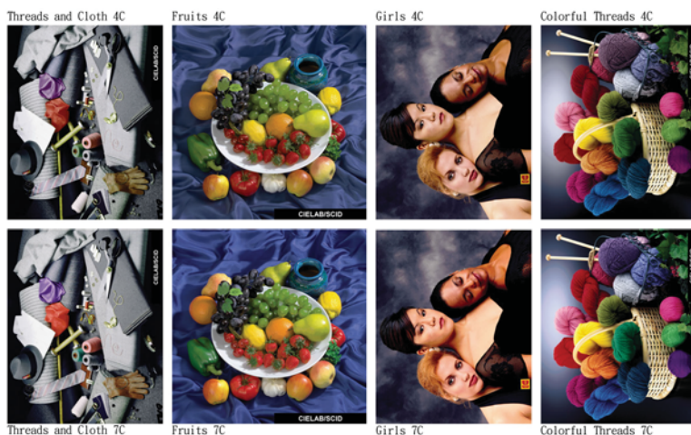
(a) Final rendition results using both processes of 4-ink (top) and 7-ink (bottom) models.
