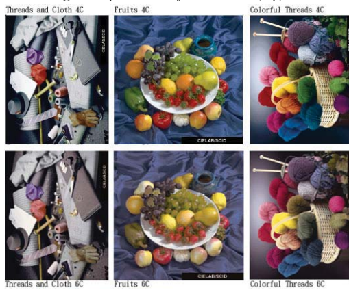
(b) Partial rendition results using both 4-colorant (top) in 4C subset and 4-colorant out of 6C superset (bottom)
