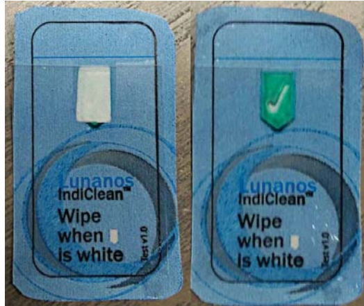
Figure 9: Prototype IndiClean Label before and after the application of cleaning solvent
