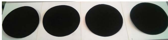
Figure 6: Conductive papers with different graphite loading
