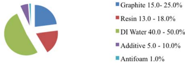
Figure 3: Composition of water based conductive ink
