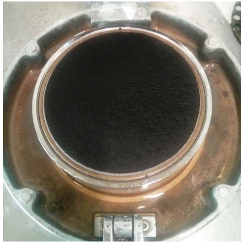
Figure 7: Formation of the graphite paper using TAPPI handsheet mold
