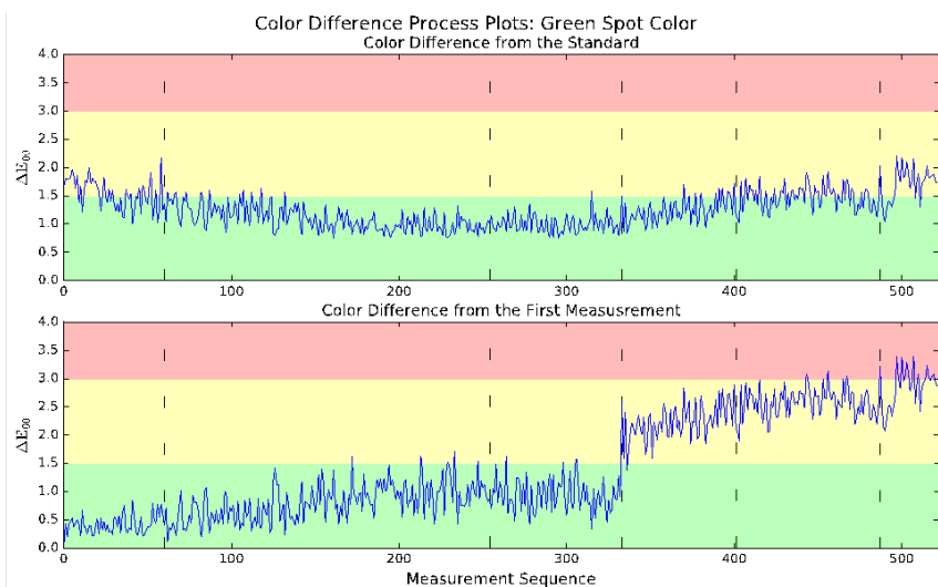
Figure 2. Color difference data process data for a green spot color. Top) Color difference from the standard, \Delta E_{00(S)} , and Bottom) Color difference from the first measurement, \Delta E_{00(D)} .
